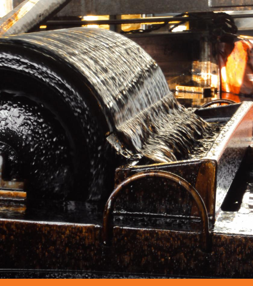
COATED DRUM SKIMMER BEING TESTED WITH DIESEL OIL
